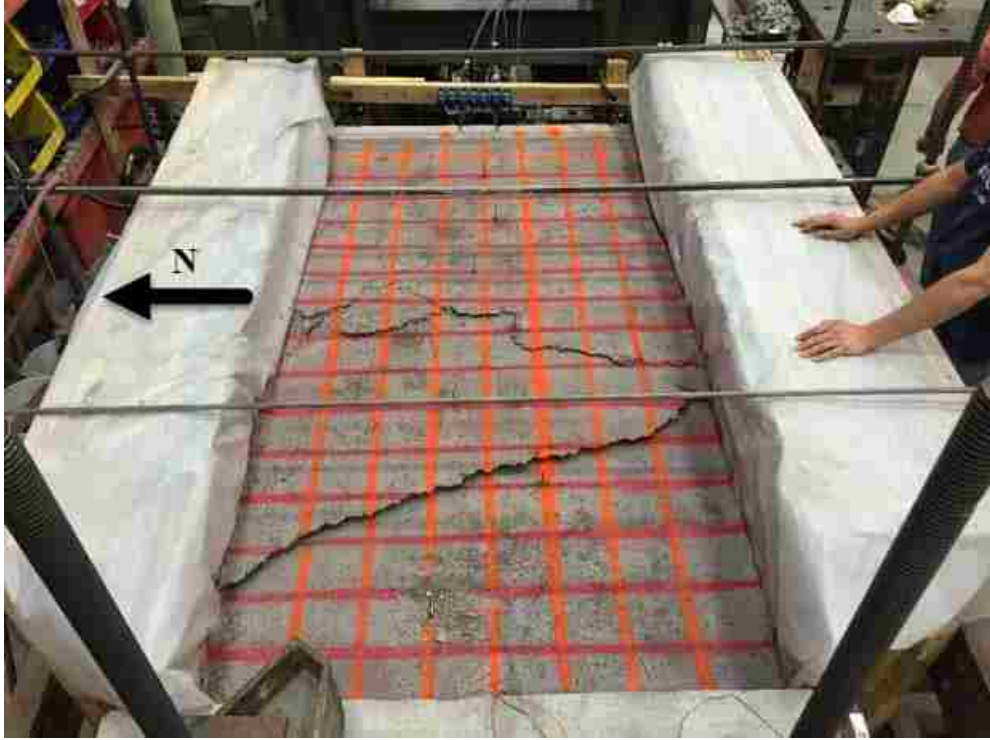
Figure 4-9. Failure surface geometries at ground surface for 0° skew test.
