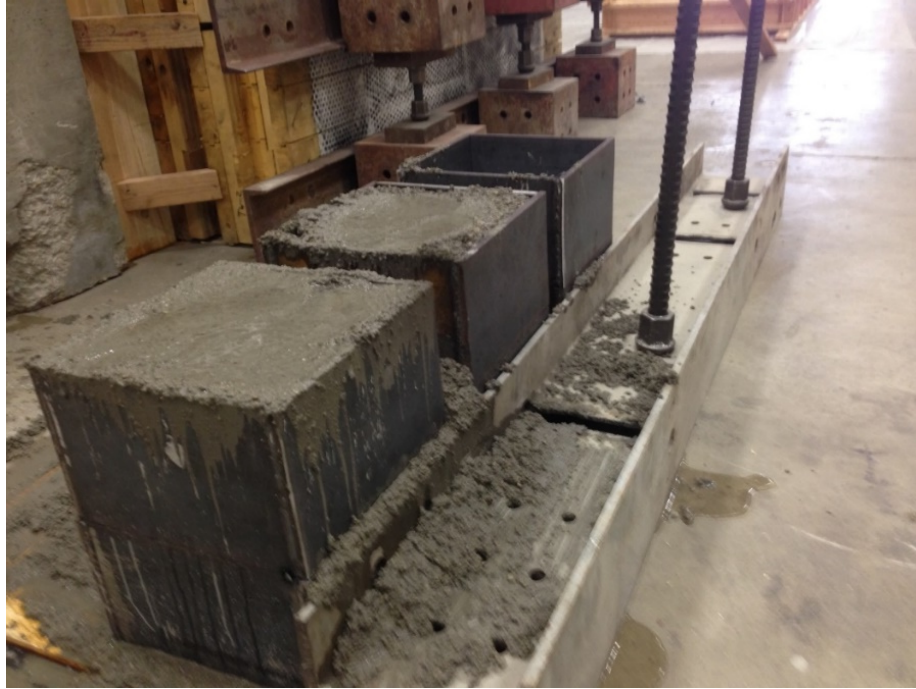
Figure 3-12. CLSM being poured into direct shear boxes.
