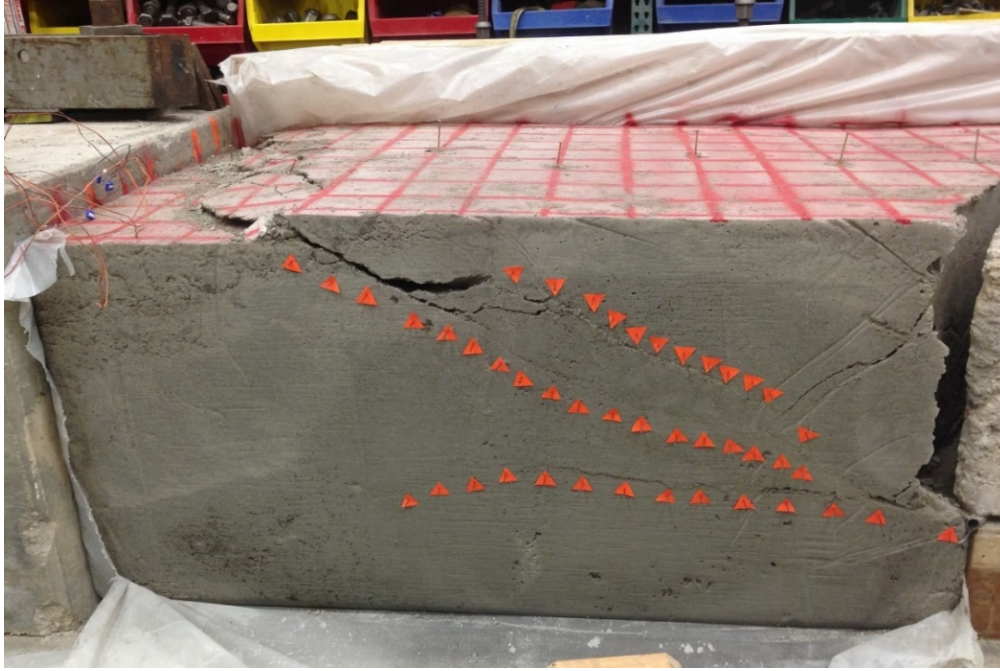
Figure 4-12. Highlighted failure planes.
