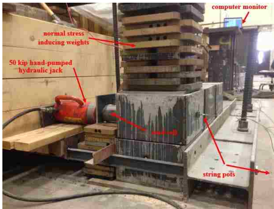
Figure 3-13. Direct shear test set-up.
