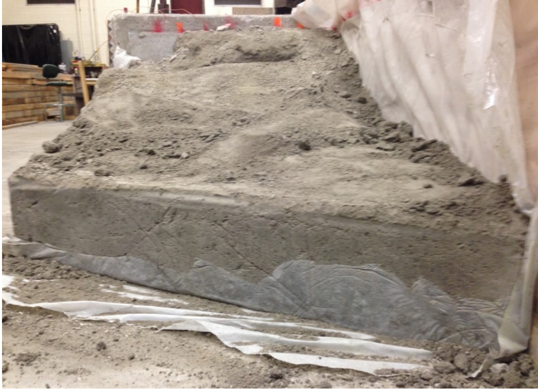
Figure 4-15. Photograph of the failure wedge from the front or East side.
